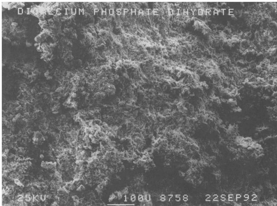
Fig. 6. Scanning electron micrographs of failure planes of tablets compacted at 10 kN from a fraction (250–300 \mu\text{m} ) of dicalcium phosphate dihydrate. Tablets were compacted from fractions lubricated with 1% magnesium stearate.
